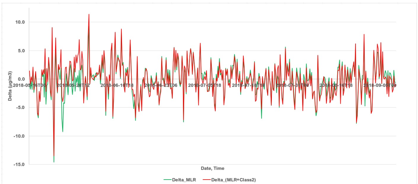
Figure 41: Difference PM2.5 versus BAM1020 for MLR, (MLR+Class2) for PMSA003_8F33 Validation Set
